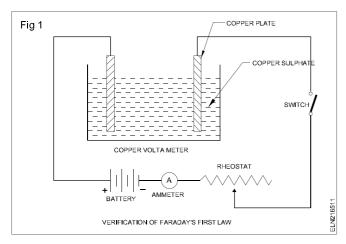
The negative elecrode is dried and weighed. After passing a definite amount of current (which can be adjusted by the rheostat) for a definite time, the cathode is weighed again, after being dried once again.
