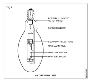
This lamp, once switched off, will not restart again until the pressure developed inside the tube falls back. It takes about 7 minutes to start again. There is no harm in keeping the switch on. The lamp should always be hung vertically, otherwise the inner tube will be damaged.
