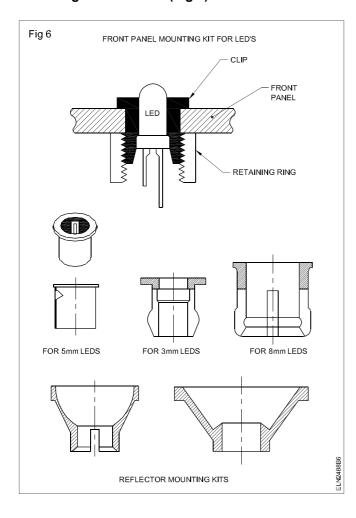
Special mounting kits Fig 6, are available for fixing the LEDs on to the printed circuit boards and monitoring panels. These kits not only extend the life of the LED by way of protecting it from mechanical stress but also make the output of the LED clearly visible.
