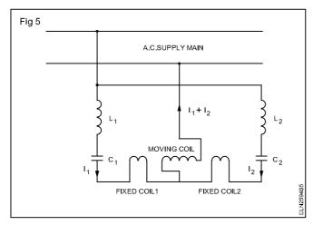
The resonant circuit of the fixed coil (1) is tuned for a frequency  $f_1$  and say 45 Hz, which is lower than the tuned frequency  $f_2$ , say, 60Hz of the fixed coil 2. The moving coil carries the vector sum of current  $\mathbf{I}_1$  and  $\mathbf{I}_2$  of the two fixed coils.
