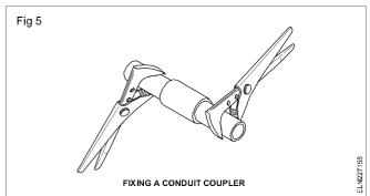
This type of running couplers makes the joint mechanically weaker and electrically non-continuous. Hence the second type of coupler uses a check (jam) nut along with the running coupler which is a much better choice than the running coupler.
