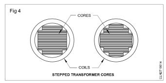
In practice, the primary and secondary windings of a transformer have two or more coils per leg. They may be arranged in series or parallel. The laminations are pressed together by clamping in such a way as to prevent any fluttering or shifting.
