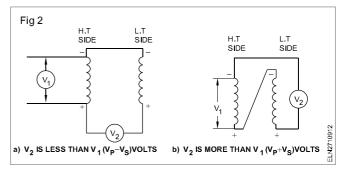
If in transformer has similar ends in one side (Fig 3a) the polarity marking is said to be subtractive polarity marking on the other hand if the opposite ends are in one side (Fig 3b) the polarity marking is called as additive polarity marking.
