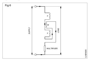
**Dynanometer used as a Wattmeter:** The dynamometer is commonly used as a wattmeter to measure power in both AC and DC circuits and will have uniform scale.
