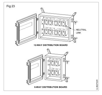
**Neutral link:** In a three-phase system of wiring installations, the phases are controlled through switches, and the neutral is tapped through a link called neutral link. The neutral link consists of a terminal for incoming current and a multi-way outgoing circuit. The metal terminals are mounted on high grade vitreous porcelain base (Fig 24). The ratings are 16A, 32A, 63A, 100A neutral link.
