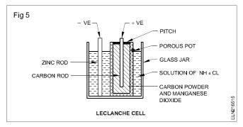
**Dry cell** (Carbon-Zinc cell): The danger of spilling the liquid electrolyte from a Leclanche type of cell led to the invention of another class of cells called dry cells.
