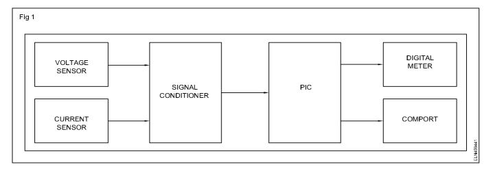
The voltage sensor built around a step down element and potential divider network sensors both the phase voltage and load voltage.
