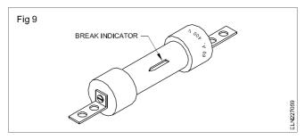
Normally a silver alloy is used as the fusing element and when it melts due to the excessive current, it combines with the surrounded sand/powder, and forms small globules without making an arc, spark or gas. HRC fuses can open a short-circuited circuit within 0.013 second. It has an indicator to show the fuse has blown. The rupturing capacity of the fuse could be calculated from the following formula.
