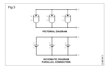
Identical cells are connected in parallel to obtain a higher output current or ampere-hour rating. With this connection of cells, the output ampere hour rating is equal to the sum of the ampere hour ratings of all the cells. However, the output voltage remains the same as the voltage of a single cell.
