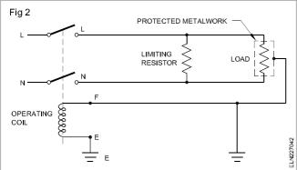
Voltage operated ELCBs are meant to be used where it is not practicable to meet the requirements of IEE wiring regulation by direct earthing or where additional protection is desirable.
