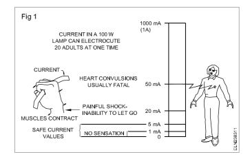
Reasons for earthing: The basic reason for earthing is to prevent or minimize the risk of shock to human beings and livestock. The reason for having a properly earthed metal part in an electrical installation is to provide a low resistance discharge path for earth leakage currents which would otherwise prove injurious or fatal to a person or animal touching the metal part.
