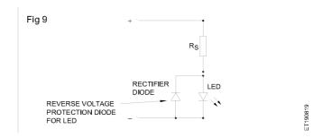
In Fig 9, when a reverse voltage across the LED becomes more than 0.7 V, the rectifier diode conducts with a forward voltage of 0.7 V. Thus the reverse voltage across the LED is restricted to 0.7 V which is much less than the maximum reverse voltage of 8 V of the LED, and hence the LED is safe.
