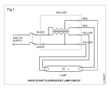
Since the cathodes are already heated, the amount of voltage required to cause the lamp to fluorescent is smaller than the voltage required for the instant start lamp. As a result, the rapid start system is very efficient particularly because of the small amount of loss in the ballast.
