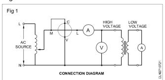
The low voltage side of the transformer is short circuited. A reduced voltage applied on the high voltage winding of the transformer such that the rated current flows through the ammeter. In this condition the impedance of the transformer is merely as equivalent impedenence (Fig 2).
