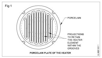
Porcelain withstands high temperature and remains as a good insulator even at high temperatures, say 1300°C. The coiled Nichrome heating element is housed in the grooves. The grooves are designed with projections at various places (Fig 1). The projections prevent the heating element from coming out of the grooves.
