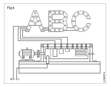
**Electrical motor:** A single phase, low speed motor usually the shaded pole motor with sufficient power to drive the drum, is used for this purpose.
