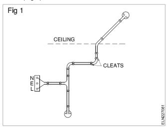
Cleat wiring is recommended only for temporary installations. These cleats are made in pairs having bottom and top halves (Fig 2). Bottom half is grooved to receive the wire and the top half is for cable grip.
