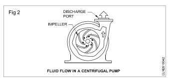
The operation of a centrifugal pump is based on centrifugal force. As the fluid being pumped enters the inlet or central section of the pump, the rotating action of the impeller vanes forces it to the outside of the pump casing (Fig 2).
