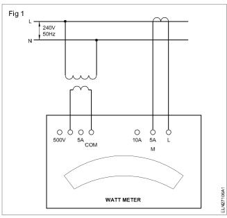
The maximum dial reading (Full scale deflection FSD) indicates 625 watts. Find the meter constant and actual power if the meter reads 600 watts against the following ranges.
