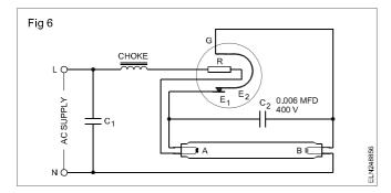
A 0.006 MFD capacitor ( $C_2$ ) is connected across the electrodes of the starter contacts (bimetals) in the case of both thermal and glow type starters, to eliminate any radio interference effects that may be caused by the opening and closing of the bimetallic contacts.
