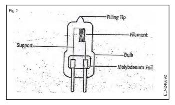
To maintain this regenerative cycle, it is necessary that the wall temperature is maintained high to 2500°C. The lamp envelope is therefore made of quartz due to which it is possible to miniaturise, as filling gas can now be filled at high gas pressure.
