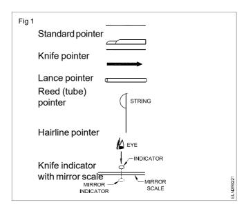
Due to the gap between the pointer and the scale, while reading an instrument, a slanting view may be obtained. Depending on the eye angle, a reading error may exist. This error is known as parallax error.
