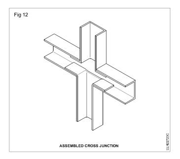
Attachment of cover: Cover should be attached to channel in individual sections after drawing all wires inside. No screws or nails shall be used for fixing PVC capping (cover) to the casing (channel). The capping (cover) should be slided in through the grooves. Metallic capping (cover) shall be fixed by using cadmium plated screws in a staggered manner with axial spacing not exceeding 30cm.
