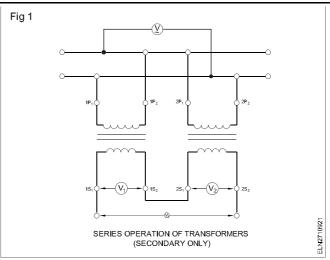
In series operation, individual secondary voltages of both transformers are added if they are connected with proper polarity, but the current ratings are remains same.
