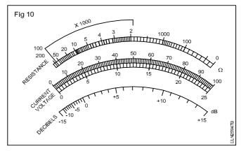
The scale of current and voltage is uniformly graduated.
