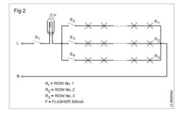
The rating of the flasher in each row of (small) low voltage lamps must be the same as that of the other lamps in that series circuit. If the lamps are of different ratings, then the flasher should be of the lowest current capacity in that circuit
