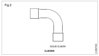
The axis of any elbow shall be a quadrant of a circle plus a straight portion of each end. Elbows are used at sharp ends of nearby walls or roof and wall.
