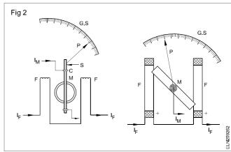
**Working:** As shown in Fig 3,let the current passing through the fixed coils be  $I_F$ , and the current passing through the moving coil be  $I_M$ . The field strength will be proportional to the current  $I_F$ .
