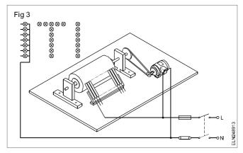
The length of the drum is determined by the number of finger-strips, and the diameter of the drum depends on the number of circuits to be incorporated. The speed of the drum must be as low as possible which is obtained by using two pulleys of different sizes to create a high ratio. (Fig 3) The drum-plates are usually made of brass/copper, and are nailed. The contact strips are fixed by screws or wire nails. (Fig 4)
