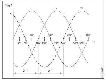
Importance of correct phase sequence: Correct phase sequence is important in the construction and connection of various three-phase systems. For example, correct phase sequence is important when the outputs of three-phase alternators must be paralleled into a common
