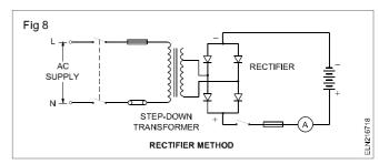
**Trickle charge**: When the battery is charged at a very low rate, that is 2 to 3% of the normal rate for a long period, it is said to be a trickle charge.
