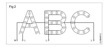
Mark the lamp position on the layout, connect all the lamps in parallel of letters A, B and C as shown in Fig 2, and then test the lamps for each letter by effecting supply. The neutral is run to all the lamps commonly.
