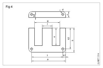
The nearest size sheet should be selected from the standard size of the stamping table. Here we assume the centre limb width to be 20 mm, and hence, the core E.I. 60 is selected. However, you may select any other type to suit the cross-section. But the other details like the number of stampings and the bobbin dimensions may change accordingly.
