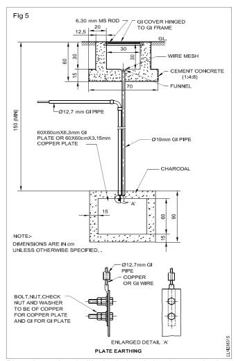
Plate electrodes shall be buried such that the top edge is at a depth not less than 1.5 m from the surface of the ground.
