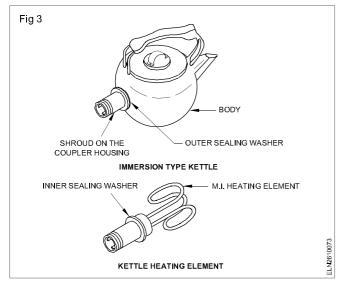
New elements can be fitted to most types of kettles without difficulty.
