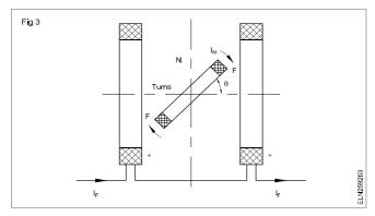
The deflecting torque is produced due to the interactions of the magnetic fields produced by the fixed and moving coils and will be proportional to the current carried by them.
