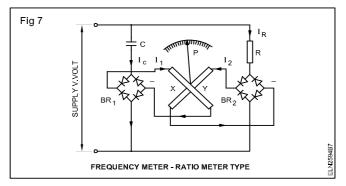
**Working:** The current through the coil depends upon the supply frequency. At higher frequency, the current through the coil X is higher whereas the current through coil `Y' is independent of the frequency. The torque developed in the coil depends upon the interaction between the permanent magnetic field and the resultant field created by the coil currents.
