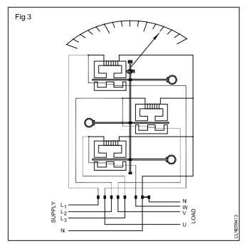
The principle and working of an induction type wattmeter are similar to the induction type energy meter. The only difference in construction between the energy meter and wattmeter is that the spindle of the wattmeter is spring-controlled, has a pointer but no train of gears.
