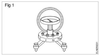
**Secondary instruments:** In these instruments the value of electrical quantity (voltage, current, power, etc.) to be measured can be determined from the deflection of the instruments on the calibrated dial. These instruments should be calibrated in comparision with either an absolute instrument or with one which has already been caliberated. All the instruments used commercially are secondary instruments.
