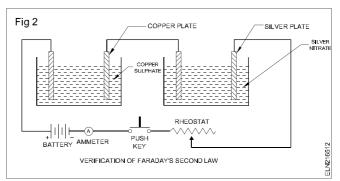
Now a definite current is passed for a definite time through both the voltameters. If the mass of copper deposited at the copper cathode is  $m_1$  and the mass of silver deposited at silver cathode is  $m_2$  and their chemical equivalents are  $w_1$  and  $w_2$  respectively, then it is found that -
