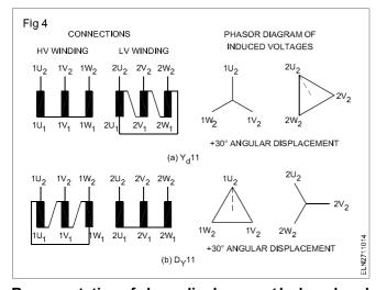
**Representation of phase displacement by hour hand of a clock**: The phase difference between the HV and LV windings for different types of connections can be represented by comparing it with the hour hand of a clock.
