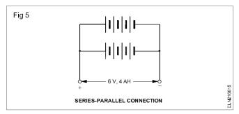
The number of cells that must be connected in series to have voltage rating is calculated first and then the number of parallel rows of series connected cells is calculated for required ampere-hour rating.
