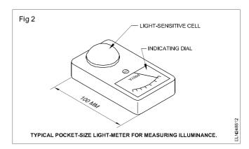
Measured brightness is termed `luminance', and it should not be confused with `illuminance'. Luminance is the lumens emitted by a luminous surface of one square metre.
