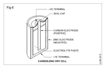
As with all primary cells, one of the electrodes becomes decomposed as part of the chemical reaction. In this cell the negative zinc container electrode is the one that is used up. As a result, cells left in equipment for long periods of time can rupture, spilling the electrolyte and causing damage to the neighbouring parts.
