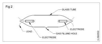
The length of the tube varies from 1 metre to 5 metres, and the diameter varies from 10 mm to 20 mm. The tubes are joined with electrodes which are operated at high voltage. The electrodes are connected with nickel wires for more length or to different letters. (Fig 3)
