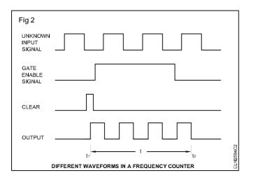
After  $t_2$ , the AND gate output will be again LOW and the counter will stop counting. Thus, the counter will have counted the number of pulses that occurred during the time interval, t of the GATE ENABLE SIGNAL, and the resulting contents of the counter are a direct measure of the frequency of the input signal
