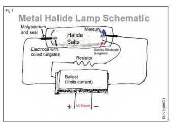
When the lamp is cold the halides and mercury are condensed on the fused quartz tube. When the lamp is turned on current passed through the starting electrode and jumps the short distance to the main electrode (Fig 1), this is aided by argon gas. The argon strikes an arc at low temperatures.
