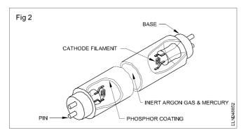
The inner surface of the tube is coated with a fluorescent powder or phoshphor. This phosphor emits light when exposed to ultra-violet rays. Cathodes or electrodes are made up of coiled tungsten filaments coated with a mixture of barium and strontium oxides.
