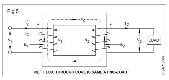
When the transformer is in no-load, the primary winding has two currents  $I_0$  and  $I_2$ . The total primary current  $I_1$  is the vector of  $I_0$  and  $I_2$ . The elementary vector diagram of
