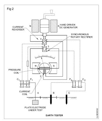
When DC is used in electrode resistance measurement the effect of electrolytic emf interferes with the measurement and the reading may go wrong. To avoid this, the supply to the electrodes should be AC.
