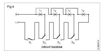
While coming back from the godown when the person switches off the light 4, then the light 3 will be on and give light for his return movement. When he leaves the godown all the lights could be switched 'off' by operating switch S<sub>1</sub>.
