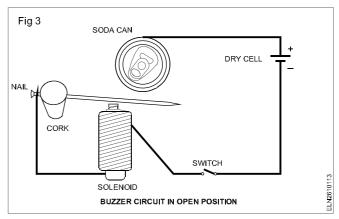
Then the circuit completes the current flow again and repeats the cycle. Each time the nail strikes back at the can, a sound is produced. Depending on the distance between the electromagnet and the nail several sound is produced.
