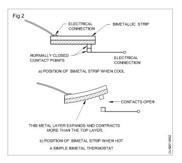
In the thermostat there is a bimetal strip made of two strips of metal with different expansion rates welded together. The metal strip expands when heated and contracts when cooled. One metal in the bimetal strip has a high rate of expansion when heated, and the other has a low rate.
