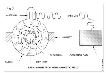
As the electrons approach the anode, they travel past the small resonant cavities to oscillate at a very high frequency of 2450 MHz. This RF energy is radiated into the cooking cavity where food is placed to be heated.
