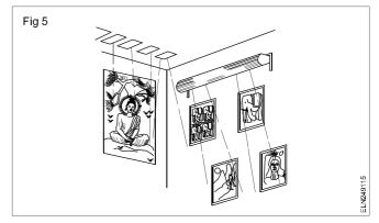
Footlight type trough lighting for counter and shelf displays ranges from single lumiline reflectors for counter cards and small displays to extended shelf troughs as illustrated. Trough footlights with changeable, luminous sign panels transform waste space into valuable display. (Fig 6)
