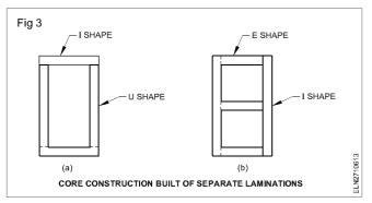
**Core construction:** As a rule, the number of butt joints is to be limited. The joints are tightly made and laminations interleaved so as to minimize the reluctance of the magnetic circuit. The stacking of laminations to the required core cross-section results in the core legs of square or rectangular cross-section. This permits coils to
