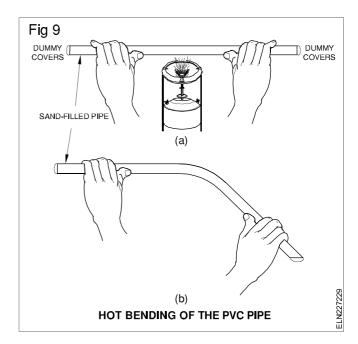
Then bend the required angle is made by holding both sides, with sufficient gap from the heated portion to avoid burning of hands, and applying uniform pressure (Fig 9b). Care shall be taken to avoid kinks on the conduits while bending.
