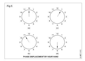
**Vector groups:** Depending on the phase displacement of the voltages of HV and LV sides, transformers are classified into groups called 'vector groups'. Transformers with the same phase displacement between the HV and LV sides are classified into one group. Various vector group arrangements used and their connections symbols are given in Indian Standard IS:2026 (PartIV)-1977.
