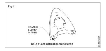
**Sole-plate:** The transfer of heat from the heating element within to the material being ironed is done by the sole-plate (Fig 4). The material being pressed can be easily damaged if the sole-plate is not smooth and free from scratches. If the sole-plates are scratched, they can be buffed and polished.
