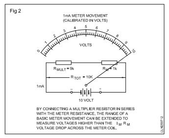
**Sensitivity of voltmeter**: An important characteristic of any voltmeter is its impedance or ohms per volt (ohms/volt) rating. Ohms/volt rating is the voltmeter sensitivity. The ohms/volt rating is defined as the resistance required  $(R_M + R_{MULT})$  for full scale deflection. For example, the 1mA 1000 ohms meter movement indicates 1 volt at full scale deflection. Therefore its `ohm/volt' rating is 1000/1 or 1000 ohms/volt (Fig 3) ohms/volt =  $E_{MAX}/I_M$ .
