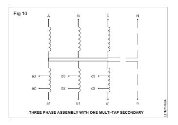
The letters A,B,C denote fully insulated terminals and the letter N denotes a terminal intended to be earthed and the insulation of which is less than that of the other terminals.
