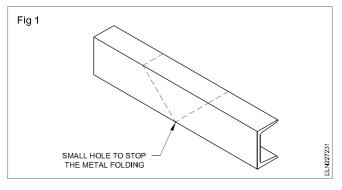
3 Place wood blocks inside trunking for support. Cut sides of trunking (Fig 2).
