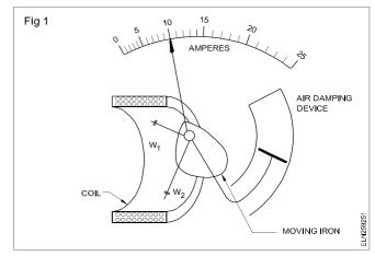
When the electromagnetic coil is connected to the supply, the magnetic field created in the coil attracts the soft iron piece (Fig 2). Due to the eccentricity of pivoting of the iron piece, the enlarged portion of the iron piece is pulled towards the coil. This in turn moves the spindle and makes the pointer to deflect.
