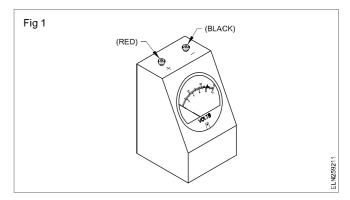
In the moving iron type there is no polarity marking on the terminals. Both the terminals are of the same colour. The instrument can be connected in the circuit without identifying the line and neutral of the supply.
