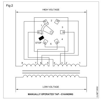
There are two methods of tap changing. In one method, these taps are manually changed through a tap changing switch. (Fig 2) In this method load switch has to be opened, before the tap changing operation is to avoid heavy sparking at the contact points. This method is often referred to as "OFF-LOAD" tap changing method.
