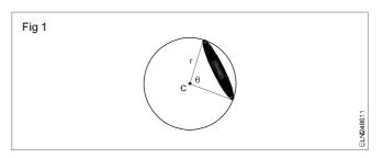
If the shaded area =  $r^2$  and a source of one candela is at the centre C, the light contained within the solid angle is one lumen.
