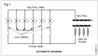
In domestic wiring installation, the looping-back system should be preferred.
