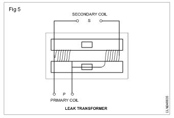
The device now acts as a choke coil reducing the voltage across the lamp electrodes to the required value.
