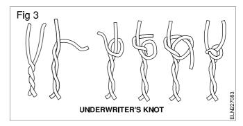
A knot is made on twin-twisted or twin-core flexible cable inside the accessories' cap cover.
