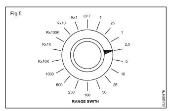
a meter having the function and the range selected by a single switch.
