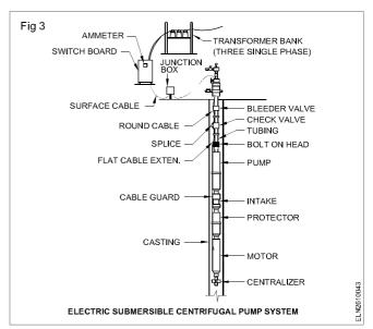
**Submersible pumps**: This pump also comes under the category of centrifugal pumps and is found in use at places where water is found in great depth.
