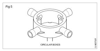
Small circular boxes shall be provided with two machine screws of a diameter not less than 2.8 mm for fixing the covers. Large circular boxes have four machine screws of not less than 4 mm diameter having not less than 10mm threaded portion for fixing the cover.
