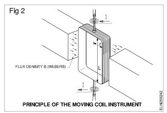
The current in amperes passing through the coil and N is the number of turns.
