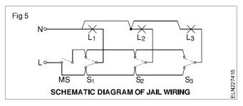
The master switch (MS) could be operated by the warden to make all the lights ON when they are all OFF.
