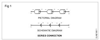
Identical cells are connected in series to obtain a higher voltage than is available from a single cell. With this connection of cells, the output voltage is equal to the sum of the voltages of all the cells. However, the ampere hour (AH) rating remains equal to that of a single cell.
