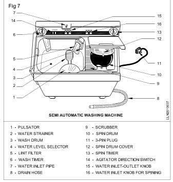
speed and due to centrifugal action the water from the clothes is removed fully till it is just damp dry. The time duration spin operation may be manual or automatic with the help of a timer depending upon the model.
