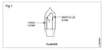
When the row of lamps is connected across the supply and switched ON, the bimetal strip gets heated up, this breaks the contacts and disconnects supply to the other lamps, making the lamps OFF.
