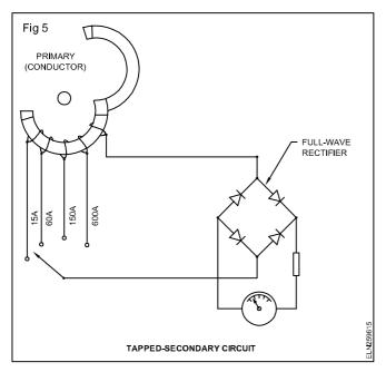
**Safety:** The secondary winding of the current transformer should always be either shunted or connected to the ammeter; otherwise, dangerous potential differences may occur across the open secondary.
