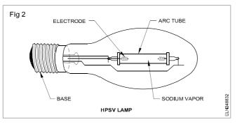
This discharge tube is made of sintered aluminium ceramic discharge arc tube which is resistant to the hot ionised Sodium Vapour up to a temperature of about 1600°C which transmits over 90% of visible radiation.
