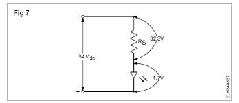
For the LED to give reasonably good light, the current through the LED has to be 20 mA, as indicated in the specifications sheet. So, the value of  $R_{\rm s}$  must be,
