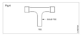
Tees are used to take diversion from the main line either to the switch points or the light points. It may be either an ordinary type or an inspection type. Inspection type tees are used to assist in the inspection in case there is a need.
