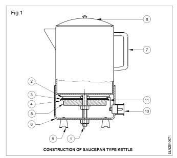
**Asbestos sheet:** This is placed below the element and mica insulation to serve as a heat insulator. It reduces the heat loss in the kettle in addition it gives increased insulation.
