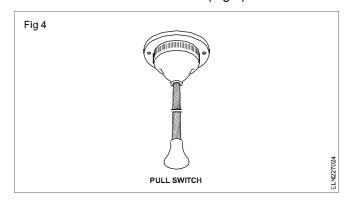
This switch is mounted on ceilings. As the user could operate the switch from a distance through the insulated cord, this could be used safely for operating water heaters in bathrooms or fan or lights in bedrooms.
