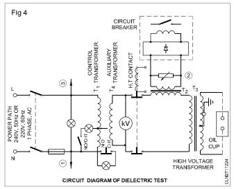
For conducting dielectric test on transformer oil, the oil is to be gently agitated and turned over several times so that homogeneous distribution of the impurities contained in the oil is spread all over.
