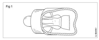
This type of construction results in lower electrode losses. The other details of construction for instant start fluorescent tubes are the same as for preheat fluorescent tubes with the exception that the diameter of the instant start tubes is slightly smaller than that of the pre-heat fluorescent tubes.
