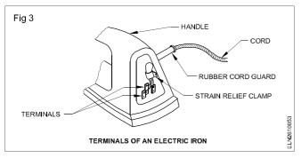
Handles: Handles are made of wood or plastic. In modern irons, plastic handles are made in large units combining the handle and brackets in a single unit mounted directly on the cover. Sometimes handles are split to provide access to the terminal covering and an entrance for the cord. When disassembling an iron for repair, the handle and its part are usually the first to be disassembled.
