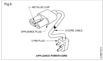
For this the appliance plug has two spring-loaded, metallic clips on either side of it which makes the contact with metallic enclosure of the socket when plugged. As rusting prevents proper contact of these clips with the socket, for safety, these clips and sockets are made of nickel-plated brass. If the spring tension of the clip is lost, it should be replaced. Otherwise earth contact will not be proper.
