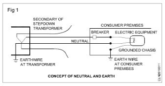
Earth point is the point connected to the ground, i.e. earthed locally at the consumer premises while Neutral point is the star point of the secondary stepdown transformer feeding the consumer premises.
