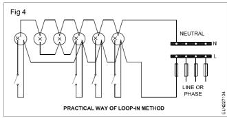
**Loop-in method by 3-plate ceiling rose:** We can also use 3-plate ceiling roses (Fig 4). Considerable cable length could be saved by using the third terminal of the ceiling rose as a looping-in terminal for the switch drop, so that two cables only are required from the ceiling rose to the switch.
