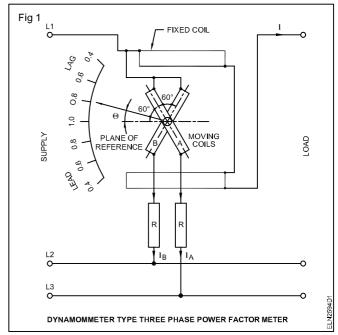
In this meter, the field coils are connected in series with the load along with one phase. The two moving coils are rigidly attached to each other at an angle of 120°. These coils are connected to two different phases. A resistance is connected in series with each coil.
