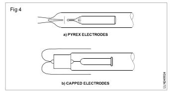
The shape of the electrode is cylindrical. The electrodes are made of nickel, iron or copper. The electrode consists of:
