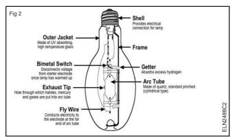
Light is generated by creating an arc between the two electrodes located inside the inner arc tube. The inner arc tube is typically made of quartz, and this is a very harsh environment, with high temperatures approaching 1000°C and pressure of 3 or 4 atmospheres.
