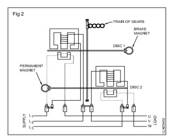
In both the cases the driving torque produced by individual elements are summed up. The recording mechanism which is attached to the train of gears i.e., cyclometer or counter type dial shows the sum of the energies that has passed through the elements. The two element energy meter is only suitable for a 3-phase 3-wire system but can be used for both balanced and unbalanced loads.
