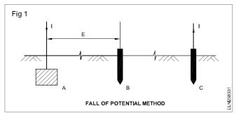
An alternating current of  $\mathbb{I}_{amps}$  magnitude is passed through the electrode A to the electrode C via the earth and the potential across electrodes A and B is measured.
