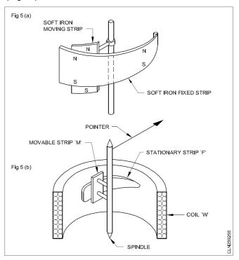
The torque, which is proportional to the square of the current, is proportionally reduced by the narrow portion of the fixed iron, resulting in more or less even torque and thereby uniform scale.
