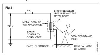
Assuming that the sum of the resistace of the main cable, metal body, earth continuity conductor and the general mass of earth is to the tune of 10 ohms
