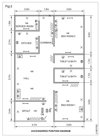
NE code recommends the horizontal run of cables should be at a height of 2.5 m (250 cm) and the height of switches from floor level should be 130 cm. The example taken here for the roof height is 3 m (300 cm) from floor level. In all cases the dimension of the rooms should be available for estimating.
