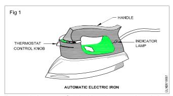
Automatic irons are fitted with a thermostatic switch to regulate the heat to a specific predetermined value. The thermostatic switch disconnects the supply when the predetermined value is reached and reconnects the supply when the iron cools down. A turning knob with a dial just below the handle, marked as rayon, cotton, silk, wool etc. can be operated to select the preset temperature.
