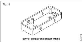
The ceiling, wall and switch boxes are normally provided with knock-out openings which can be removed when required by using punches or chisels with a stroke from a hammer. In some cases the knock-out openings could be made by the pry out-method with a screwdriver (Fig 15).
