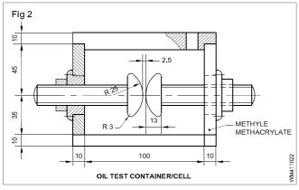
The cell shall have an effective volume between 300 to 500 ml. It should be preferably closed. Section view of container. (Fig 3)
