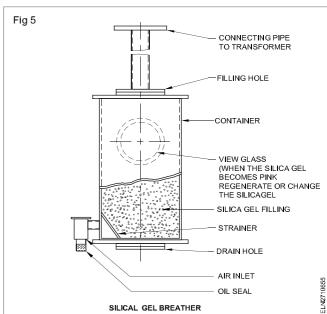
The oil seal at the bottom of the breather absorbs the dust particles that are present in the air entering the conservator.
