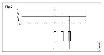
**Fuse-carrier:** The removable portion for carrying the fuse element.
