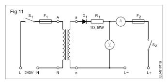
This type of circuit is protected only through fuses and needs constant attention during the entire period of battery charging. As the output voltage is fixed, only particular rated voltage batteries or a combination of them could be charged.
