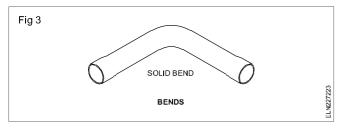
Abend gives a diversion of  $90^{\circ}$ C in the turn of a conduit, and a normal bend shall be a large sweep. Inspection type bends are used to assist in the inspection at the corners and for drawing cables.
