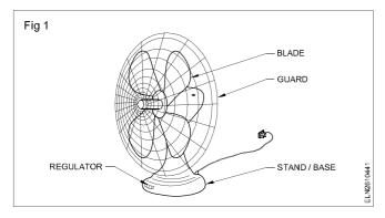
The table fan motor is mostly of a capacitor start or split phase, single phase induction type.
