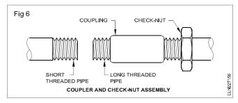
First the check-nut and then the coupler should be screwed inside the long threaded conduit. Then the short threaded conduit is butted with the long threaded conduit and the coupler is screwed on the short threaded conduit tightly.
