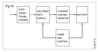
**Working**: A number of circuits are available for battery chargers. Anyhow only the 3 most commonly used circuits are explained here.
