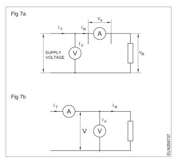
In both the cases, if readings of the ammeter and voltmeter are taken, then the measured value of resistance is given
