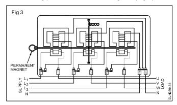
The three elements can also have a common spindle with three individual discs and braking magnets (Fig 4). Here also the 2nd type is usually preferred by manufacturers due to the easiness in construction. The driving torque produced by the three individual elements are summed up and the recording mechanism shows the sum of energies that has passed through the individual elements. This energy meter is suitable for the 3-phase 4-wire system.
