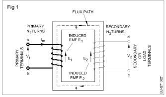
The applied voltage causes a small current to flow in the primary winding. This no-load current is meant to build up a counter-electromotive force equal and opposite to the applied voltage.
