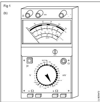
A multimeter uses a single meter movement (Fig 2), with a scale calibrated in volts, ohms and milliamperes. The necessary multiplier resistors and shunt resistors are all contained within the case. Front panel selector switches are provided to select a particular meter function and a particular range for that function.
