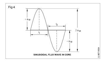
$$E_{avg} = turns \times \frac{change in flux in a given time}{given time}$$
