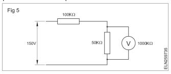
The total resistance of the circuit will be 147.6k ohm (Fig 6).
