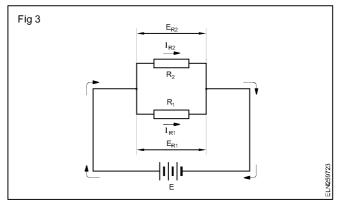
Since the same voltage appears across  $R_1$  and  $R_2$  then  $E_{R1} = E_{R2}$ . From this we derive  $I_{R1}R_1 = I_{R2}R_2$ . This equation can be used to calculate the shunt needed for a particular current measurement.
