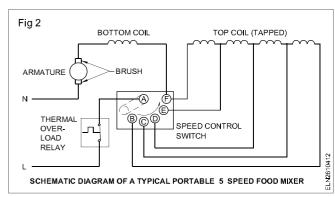
Maintenance and servicing of a food mixer: The manufacturer's service manual, if available, read it a number of times and follow the instruction. First listen to the complaint from the customer and make a note of it. Visually check the mixer right from the plug to the speed selector switch connections and enter the details in the maintenance card.
