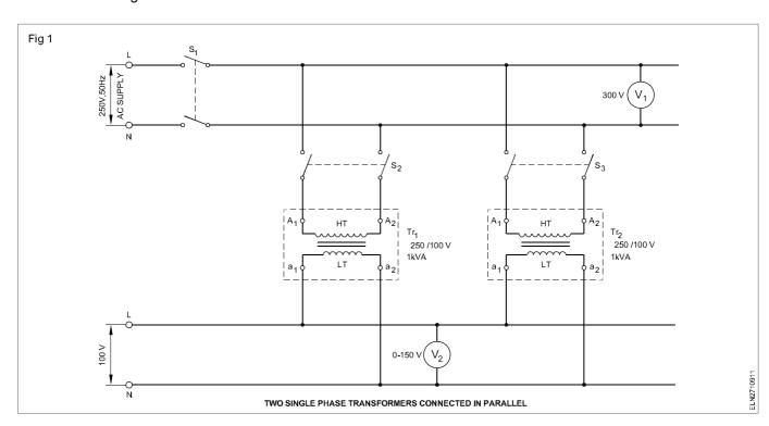
**Voltage ratio:** If voltage readings on the open secondaries of various transformers, to be run in parallel, do not show identical values, there will be circulating currents between the secondaries (and therefore between primaries also) when the secondary terminals are connected in parallel. The impedances of transformers is small, so that a small percentage voltage difference may be sufficient to circulate considerable current and cause additional I<sup>2</sup>R loss.
