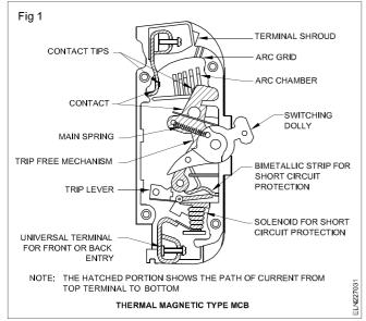
The electric current gets through two contact tips one each on moving and fixed contact of silver graphite.
