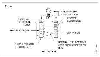
The electric current will flow as long as the chemical action continues. In this type of cell the zinc electrode is eventually consumed as part of the chemical reaction. The voltaic cell is also known as a wet cell because it uses a liquid solution for the electrolyte.
