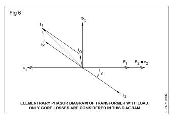
**Leakage fluxes:** When a current flows in the secondary winding, the resulting mmf  $(N_2 I_2)$  creates a separate flux, apart from the flux  $f_c$  produced by  $I_o$ , which links the secondary winding only. This flux does not link with the primary winding and is therefore not a mutual flux.
