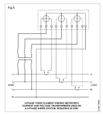
Tri vector meter is an instrument used to measure the energy used by the load in terms of KWH, KVARH, MD and KVAH.
