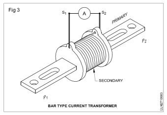
**Dry type current transformer**: This is one which does not require the use of any liquid or semi-liquid material for the purpose of cooling.
