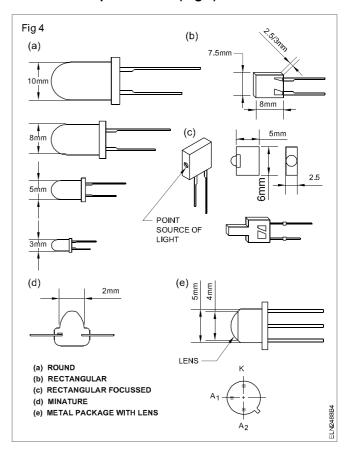
LEDs are available commercially in different shapes and sizes to suit varied commercial applications. Fig 4 shows some of the most popular shapes and sizes of LEDs.
