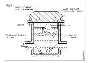
On hearing the alarm sound the operator takes necessary preventive steps to safeguard the transformer.
