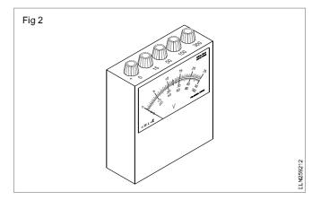
A range selector switch is used in some meters (Fig 3). While reading such meters, care should be taken to keep in mind the position of the range selector switch, and read the scale reading corresponding to that selected range.
