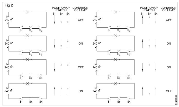
To control a lamp from three locations, three intermediate switches instead of a two two-way switches can also be used. (But, in practice, they are not used since it is very expensive).
