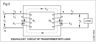
The marked terminals have the same polarity. Thus when the load is connected to the secondary, the instantaneous load current is in the direction shown.
