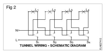
In tunnel wiring a person walking along the tunnel can successively light behind two lamps ahead and put off a lamp behind with one switch.
