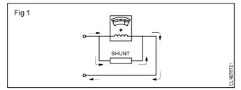
The shunt, therefore, makes it possible to measure currents much greater than that could be measured by the basic meter alone.
