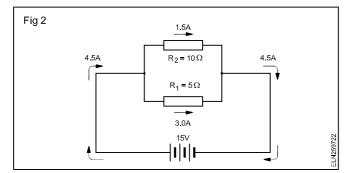
Current flow divides between two resistors parallel in a ratio inversly proportional to their resistance.
