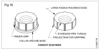
second purpose is to give a proper grip mechanically and make the conduit electrically continuous in the installation.
