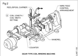
Coil length setting or layer width setting: To wind the coil of a designated length i.e. within the inner length of the bobbin two latches are provided on the transverse pulley mechanism to stop and reverse the feed at the desired point (Fig 3).
