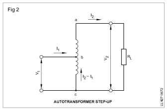
where  $N_{\rm bc}$  and  $N_{\rm ac}$  are the number of turns on the respective windings. The ratio of voltage transformation in an autotransformer is the same as that for an ordinary transformer, thus
