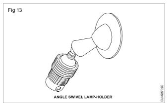
**Specification of a lamp-holder:** While specifying the lamp-holders, the type of material used for construction, type of gripping, type of mounting, working current and voltages should also be specified.
