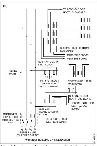
At each floor the running main is connected to the sub-main board through proper cable terminations. If there are more than one flat in each floor the individual main switches for the flat get their supply from the sub-main board through a distribution network which may include an energy meter for each flat.
