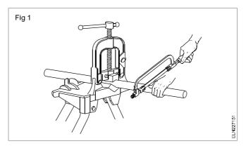
inner edge of the cut. Be sure this ridge is removed and the conduit is smooth before installing a coupling or any fitting, to avoid damage to the insulation of conductors.
