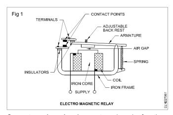
**Current sensing relay:** A current sensing relay functions whenever the current in the coil reaches an upper limit. The difference between the current specified for pick up (must operate) and non-pick up (must not operate) is usually closely controlled. The difference in current may also be closely controlled for drop out (must release) and non-drop out (must not release).
