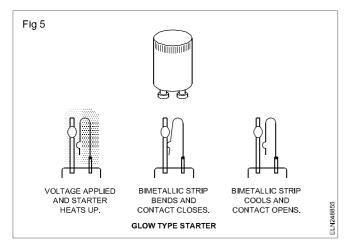
**Thermal type starter:** The switch has a bimetalic strip close to the resistance R which produces heat.
