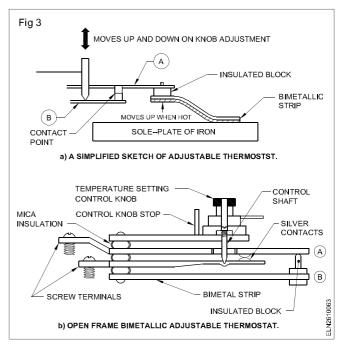
In the 'OFF' position of the temperature setting control knob, the strips A and B will be away from each other, keeping the silver contacts in an opened condition, thereby, keeping the heating element circuit open.
