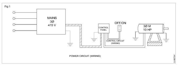
Power wiring is a high current carrying circuit which is wired to connect / disconnect the load like motors/ furnace through the protective devices like OLR and fuses etc..
