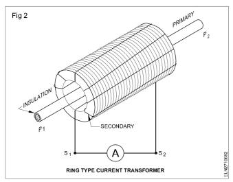
If there are 20 turns in the secondary having a current range of 5 amps, this current transformer according to the transformation ratio, could measure a primary current of 100 amps.
