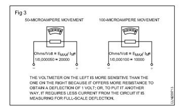
**Multi-range voltmeters**: In many types of equipment, one encounters voltages from a few tenths of a volt up to hundreds, and even thousands, of volts. To use single-range meters in these cases will be impractical, and costly. Instead, multi-range voltmeters that can measure several ranges of voltage, can be used.
