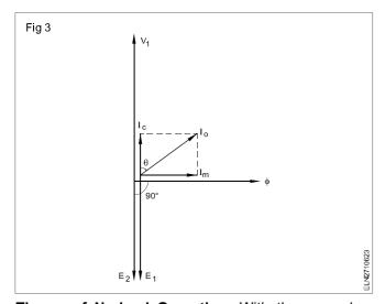
**Theory of No-load Operation:** With the secondary winding open-circuited, the no-load current  $\mathbb{I}_{\circ}$  flows in the primary winding. This no-load current has two functions:
