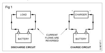
An automobile uses an automatic charging circuit as part of the car's electrical system, which is designed to recharge the battery as required and battery charging is also done using large commercial type battery chargers. Smaller type chargers are also available for use on the smaller nickel-cadmium cells. A simple variable-voltage DC power supply works well as a battery charger.
