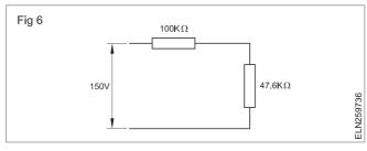
$$V_2 = \frac{47.6 \text{k ohm}}{147.6 \text{k ohm}} \times 150 \text{V} = 48.36 \text{V}$$
