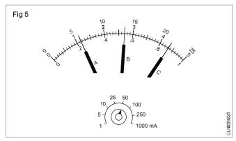
Multi-range AC/DC voltmeter scales with range and function switches set to 5V DC.
