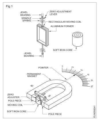
The two ends of the coil are connected to two phosphorbronze springs, fixed one on each spindle to lead in and lead out the current. The springs are spiralled in the opposite direction in order to neutralize the effect of temperature changes.
