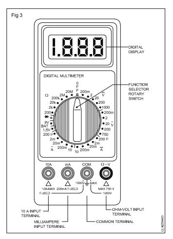
**DMM functions**: The basic functions found on most DMMs are the same as those on analouge multimeters. That is it can measure:-
