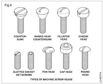
**Application:** The cheese head type of screws is used for general assembly work.
