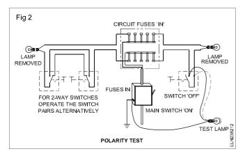
Lighting of the test lamp indicates that the phase or live cable is controlled by the switch.
