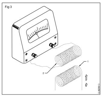
This induced emf will send the current, causing deflection of the meter. Introduction of a magnetic core between the coils increases the induced emf. The coil (1) is called primary and the coil (2) is called secondary.
