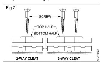
Initially the bottom and top cleats are fixed on the wall loosely according to the layout. Then the cable is drawn through the cleat grooves, and it is tensioned by pulling and the cleats are tightened by the screw.
