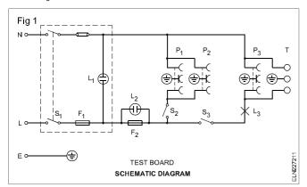
**Continuity test:** While performing a continuity test, the appliance to be tested is connected to the socket  $P_3$  or to the terminal T which are in series with the lamp  $L_3$  and are controlled by switch  $S_3$ . Normally this test is conducted by the electrician to ascertain whether the appliance is open-circuited or short-circuited. A low wattage, appliance when connected, will make the lamp  $L_3$  to burn dim, and a high wattage appliance will make the lamp to burn bright.
