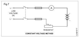
Use: For charging batteries of constant voltage rating.
