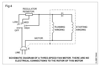
Then, if the fan motor will run only on high or medium speed but not on low speed, the problem is usually in the portion of the series resistor between the medium and low terminals. Or, if the fan motor runs only in the high position, the trouble is in the series resistance between the high and medium terminals. Also check for a dirty switch and a loose contact or wire. Often a dirty switch contact will cause one or more speeds to go dead.
